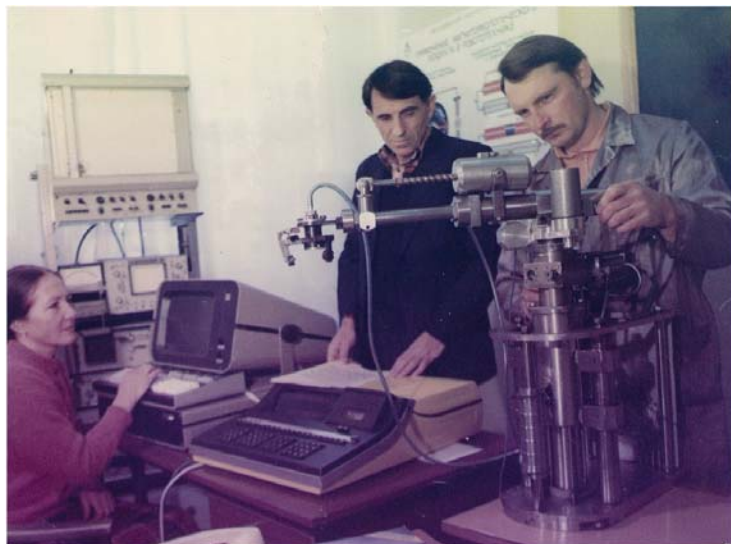
Figure 2. Prototype robot in 1986 uses MR fluid actuators. Left to right: Svetlana Demchuk, William Kordonski, Nikolai Protacevich.
