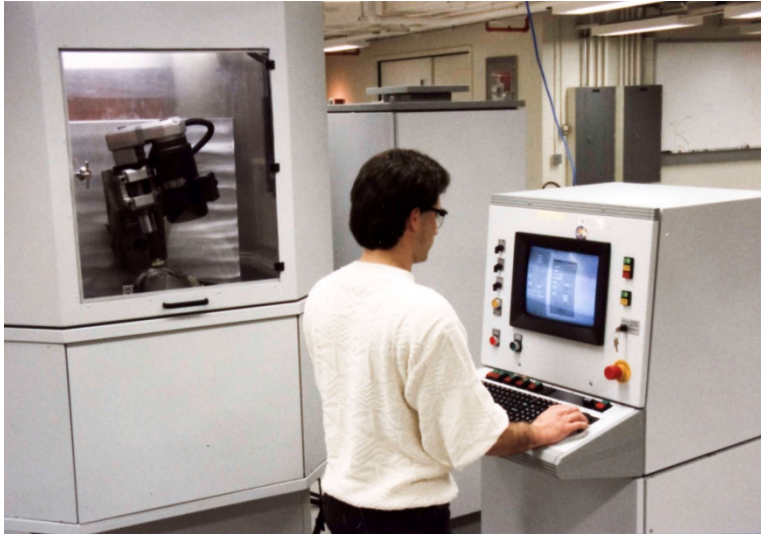
Figure 31. Left: Prototype MRF machine with vertical wheel operating at COM in March 1996 with Ed Fess at the controls. Right: Workpiece on spindle positioned over vertical wheel.
